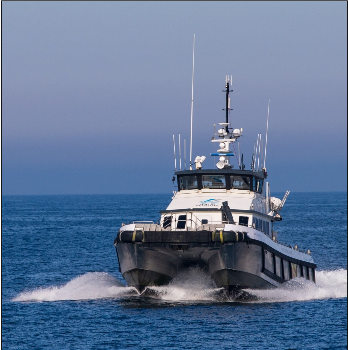
Figure 4.3132: Crew Transfer vessel (Courtesy of Beatrice OWF)
